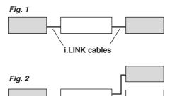
i.LINK will not work if any of the connections form a loop, as shown below.
